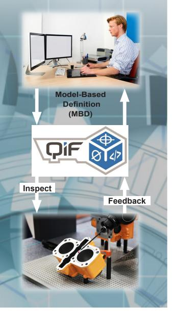
QIF is a worldwide accepted metrology standard that allows interoperability between already-in-place software and equipment, offering persistent traceability back to the CAD model
